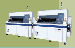
Chip mounters are used in the high-precision procedure of placing ultra-small electronic components on print substrates. These substrates, which are only a few square centimeters in size, are the central component of electronic devices such as mobile phones, digital cameras, and personal computers. Hitachi High-Tech Instruments Co., Ltd., which became a member of the Group in 2003, designs and manufactures high-speed mounter systems,
