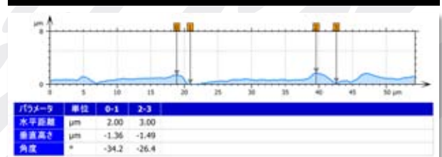
Height measurement on the extracted cross section from the 3D EDS data
