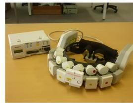
This sensor (TSND121, ATR-Promotions) was developed to measure the movement of the human body part. Data stored in internal memory were A/D-converted and transmitted to PC for analysis via Bluetooth connection. Both acceleration and angular velocity information were used for the study 2.
