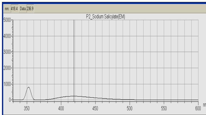
Quantum yield measurement software for simplified analysis and calculations
