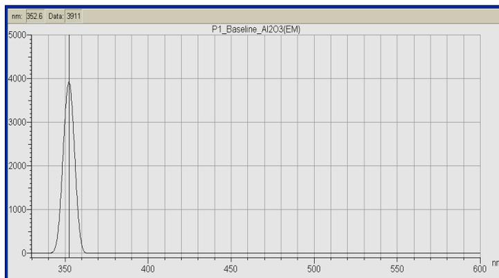
Measurement of sample (sodium salicylate), using direct excitation (Ex: 350nm).
