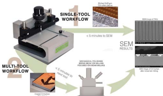
FIGURE 2. Wafers and wafer pieces enter a cross-section workflow that starts with cleaving and then follows a single- or multi-tool sample preparation process.
