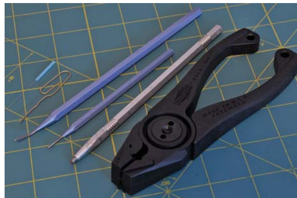
FIGURE 3a. Hand tools commonly used for cleaving semiconductor materials
