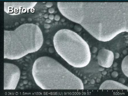
SEM Sample: PVD Tin-Gold particles
