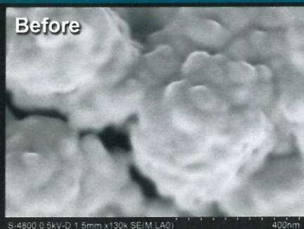
SEM Sample: Mesoporous Titanium Oxide
