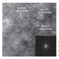
Specimen: Si single crystal Accelerating voltage:120 kV Lens mode: HR mode Magnification: ×500 k
