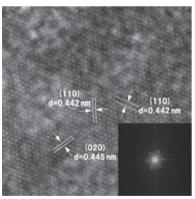
Specimen: Pyrophyllite crystal Accelerating voltage: 60 kV Lens mode: HR mode Magnification: ×400 k
