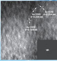
Specimen: Gold single crystal Accelerating voltage: 100 kV
