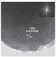
Specimen: Hydroxyapatite crystal Accelerating voltage: 40 kV Lens mode: HR mode Magnification: ×300 k
