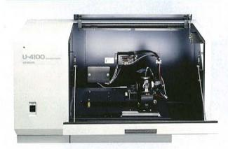
The best used as optical parts and electronics material transmittance and refrectance measurement, for instance large glass, Silicon-wafer and liquid crystal main board.
