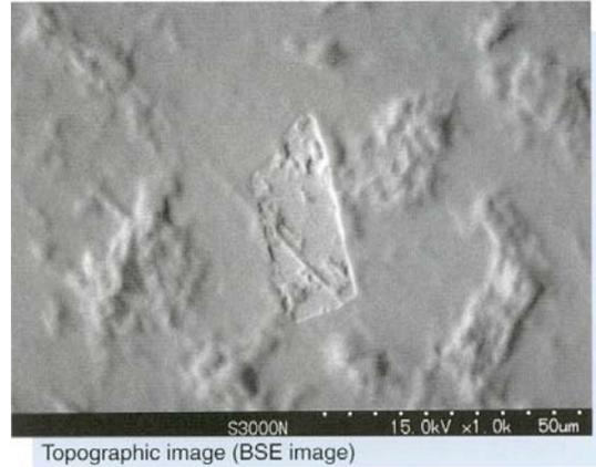
Changing the detector position permits viewing images three-dimensionally in which composition and topographic information on the specimen surface are mixed.
