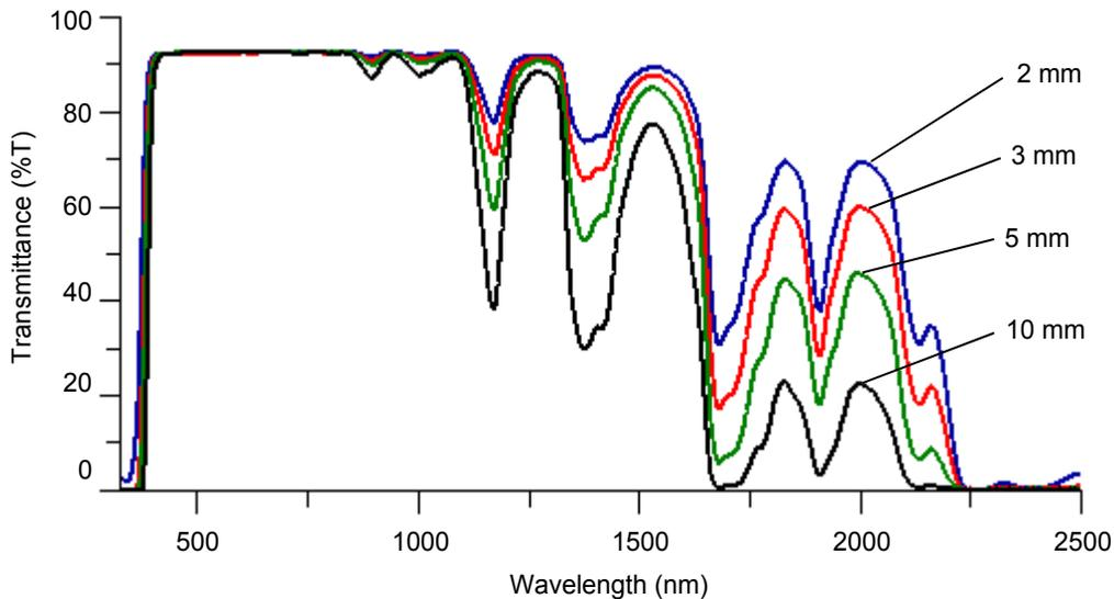
Figure 2 Transmission Spectrum of PMMA with Different Plate Thickness by UH4150
