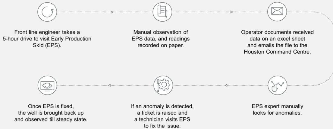
Figure 4 Initial process of anomaly detection and removal
