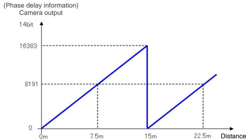
**Figure 4-1 Actual distance and depth image output value (f=10.0MHz)**
